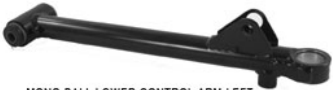
MONO BALL LOWER CONTROL ARM LEFT MONO BALL LOWER CONTROL ARM RIGHT
